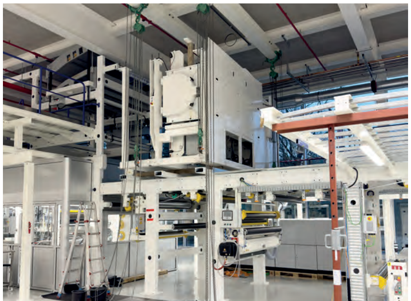
Electron beam curing unit at the new lacquer line
