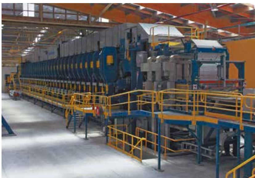
In 2006, Dieffenbacher supplied a continuous LVL-line to Pacific Woodtech. This year Roseburg Forest Products placed an order for the world's largest continuous LVL press. (Photo credit: Dieffenbacher)
